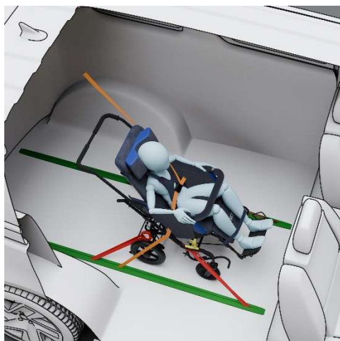
Fig. 18a Correct fastening A trolley with a patient in a vehicle
