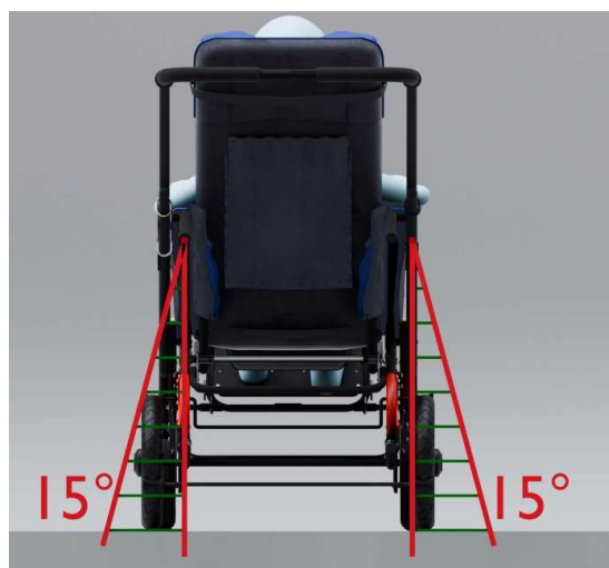
Fig. 19b Hip belt zone Rear view
